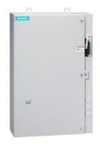
Non-reversing motor starter, Size 4, Three phase full voltage, Solid-state overload relay, OLR amp range 50-200A, 110V 50Hz / 120V 60Hz coil, Combination type, 200A fusible disconnect, 200A/600V fuse clip, Enclosure NEMA type 4/12, Water/dust tight for outdoors, Standard width enclosure
