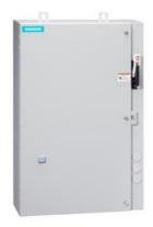
Non-reversing motor starter, Size 2 1/2, Three phase full voltage, Solid-state overload relay, OLR amp range 25-100A, Combination type, 100A circuit breaker, Enclosure NEMA type 4/12, Water/dust tight for outdoors, Extra-wide enclosure
