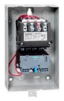
Non-reversing motor starter, Size 00, Three phase full voltage, Solid-state overload relay, OLR amp range 0.75-3.4A, 24VDC coil, Non-combination type, Enclosure type 1, Indoor general purpose use, Standard width enclosure
