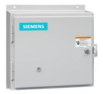
Non-reversing motor starter, Size 1, Single phase full voltage, Solid-state overload relay, OLR amp range 5.5-22A, Non-combination type, Enclosure type 12, Dust/drip proof for indoors, Standard width enclosure
