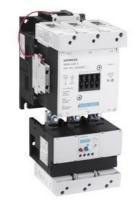
Non-reversing motor starter Size 5 Three phase full voltage Solid-state overload relay OLRelay amp range 55-250A 575-600V 50-60HZ/DC coil Combination type No enclosure
