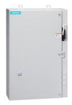
Non-reversing motor starter, Size 0, Three phase full voltage, Solid-state overload relay, OLR amp range 0.75-3.4A, Combination type, 30A fusible disconnect, 30A/600V fuse clip, Enclosure NEMA type 4/12, Water/dust tight for outdoors, Extra-wide enclosure
