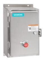
Non-reversing motor starter, Size 1, Three phase full voltage, Solid-state overload relay, OLR amp range 3-12A, 110V 50Hz / 120V 60Hz coil, Noncombination type, Encl. type 4X 304 S. Steel, Water/dust tight noncorrosive, Standard width enclosure
