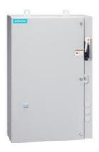
Non-reversing motor starter, Size 1 3/4, Three phase full voltage, Solidstate overload relay, OLR amp range 10-40A, Combination type, 60A fusible disconnect, 60A/600V fuse clip, Enclosure NEMA type 4/12, Water/dust tight for outdoors, Extra-wide enclosure
