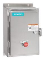
Non-reversing motor starter, Size 0, Three phase full voltage, Solid-state overload relay, OLR amp range 5.5-22A, Non-combination type, Encl. type 4X 304 S. Steel, Water/dust tight noncorrosive, Standard width enclosure
