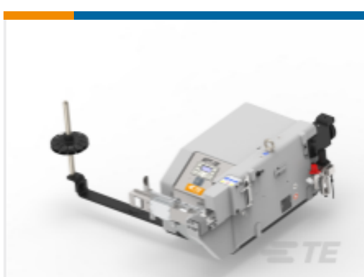
TE Part # 2161900-9 APT-5E TERMINATING MACHINE
