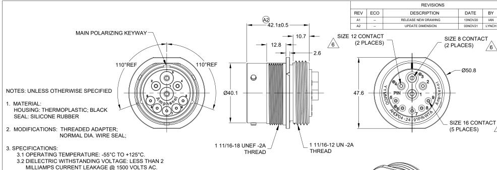
3.4 MOISTURE RESISTANCE: IP68(IM OF WATER FOR A PERIOD OF 24 HOURS, MATED CONDITION); IP69K(MATED CONDITION).
