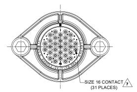
HOUSING: THERMOPLASTIC; BLACK SEAL: SILICONE RUBBER THREADED INSERT: STAINLESS STEEL
