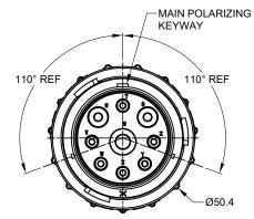
PLUG,24-09 POS, SOCKET CONT, REDUCED DIA. SEAL, AHDP
