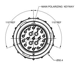
PLUG,24-21 POS, PIN CONT.,STANDARD DIA. SEAL, AHDP
