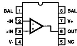
NOTE: (NC) No Connection pins may be tied to a ground plane for better isolation and heat dissipation.
