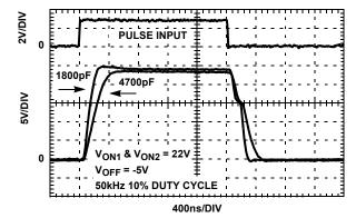
FIGURE 13. TRANSIENT RESPONSE vs LOAD CAPACITANCE
