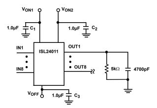
If the output load is a series  $200\Omega$  resistor and a 3300 pF then C1, C2 and C3 can be reduced to 0.47 pF.
