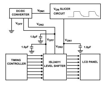
FIGURE 15. TYPICAL MONITOR APPLICATION CIRCUIT WITH SLICER TO REDUCE FLICKER
