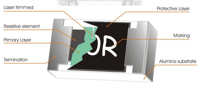
Fig 1. Construction of Chip-R
