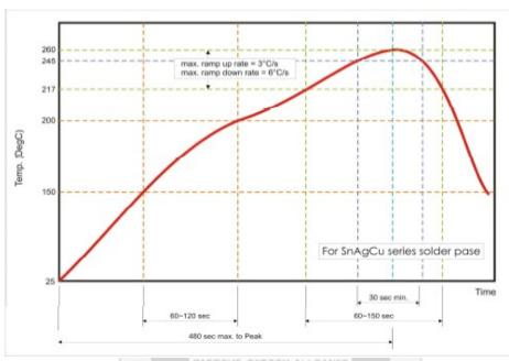
Fig 3. Infrared soldering profile for Chip Resistors
