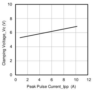
Fig3.Clamping Voltage vs. Peak Pulse Current
