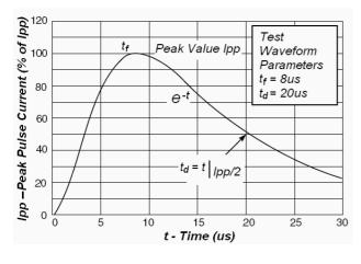
Fig1. Pulse Waveform
