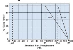
When the terminal part temperature of the resistor exceeds the rated terminal part temperature shown, the power shall be derated according to the derating curve.
