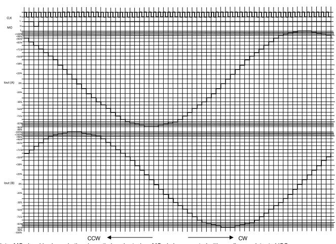
Note: MO signal is shown in the above timing chart when MO pin is connected with a pull-up resistor to VCC. Note: Timing charts may be simplified for explanatory purpose.
