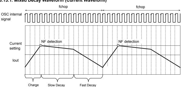
8.13.1. Mixed Decay Waveform (Current Waveform)
