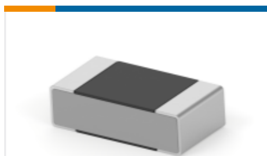
TE Part #7-1879140-3 RN 0603 105K 0.1% 10PPM 5K RL
