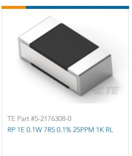
9.53  $\Omega$ , Thin Film, Precision Resistor, .1 %, 2 Termination, 0402, Taped & Reeled, .1 W, ±25 ppm/°C, Solder, Height .012 in [.3 mm], Holsworthy RP73
