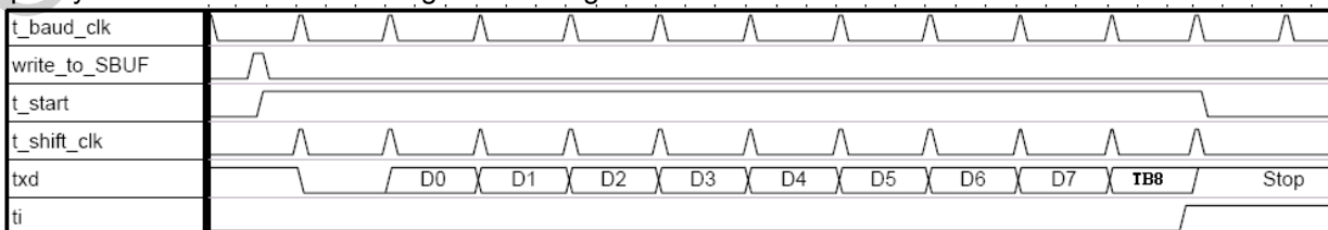
Fig. 8-5: Transmit modes 2 and 3
