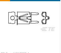
TE Part #1217080-1 FASTON 205/250 PCB MOUNTED **TPBR**
