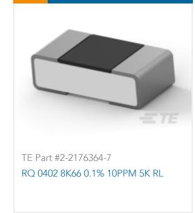
294  $\Omega$ , Thin Film, Precision Resistor, .1 %, 2 Termination, 0402, Taped & Reeled, .0625 W,  $\pm 10$  ppm/°C, Solder, Height .012 in [.3 mm], Holsworthy RQ73
