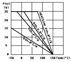
Figure 17: Maximum Allowable Power Dissipation vs. Ambient Temperature
