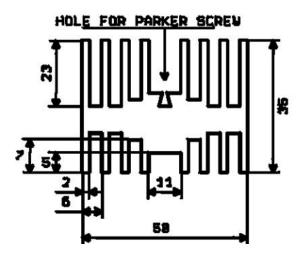
Figure 18:Example of heat-sink
