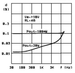
Figure 10: Distortion vs. Frequency
