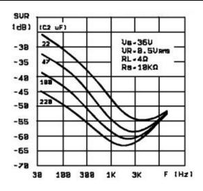
Figure 13: Supply Voltage Rejection vs. Frequency (Single
