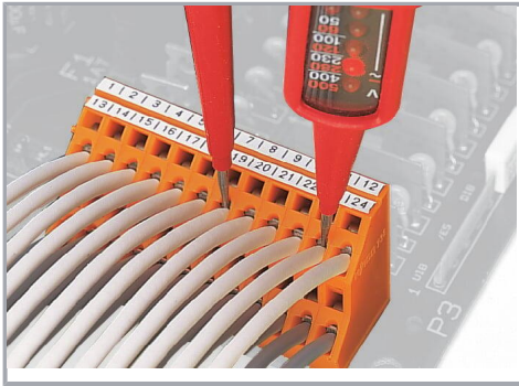
Testing via contact area above the conductors.
