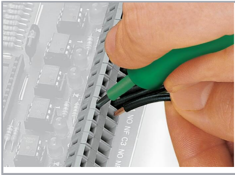
Inserting a conductor via 3.5 mm screwdriver. Screwdriver actuation parallel to conductor entry
