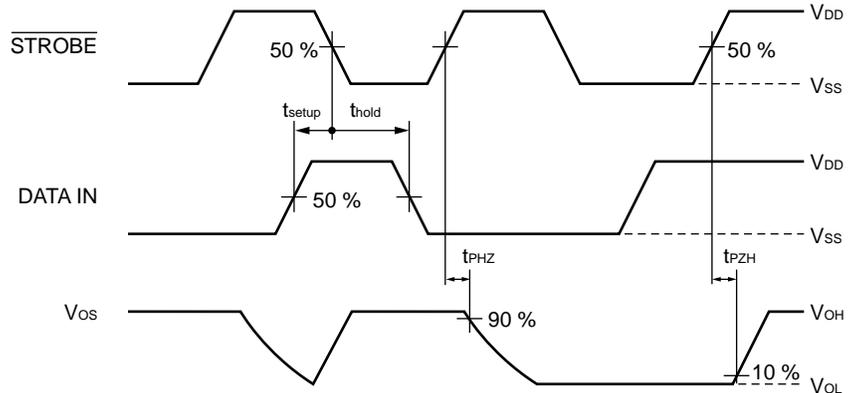
(3) DATA INPUT  $\rightarrow$  OUTPUT ( $\overline{\text{STROBE}} = V_{DD}$ )
