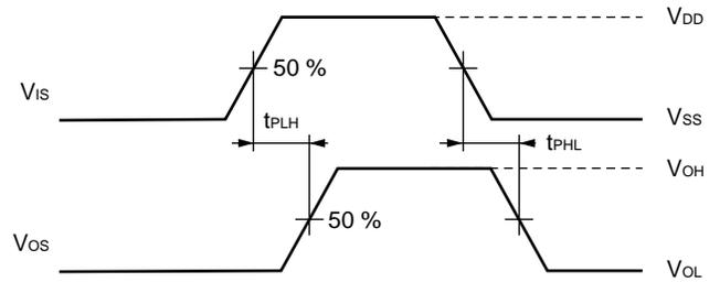
(2)  $\overline{\text{STROBE}}$  INPUT  $\rightarrow$  OUTPUT
