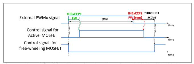
Internal signals for PWM operation - General case tON > tHBxCCP FW, tOFF > tHBxCCP Figure 27 active, motor operating as load
