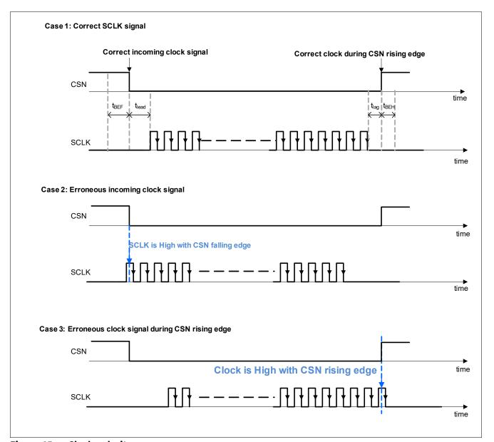
Figure 45 Clock polarity error
