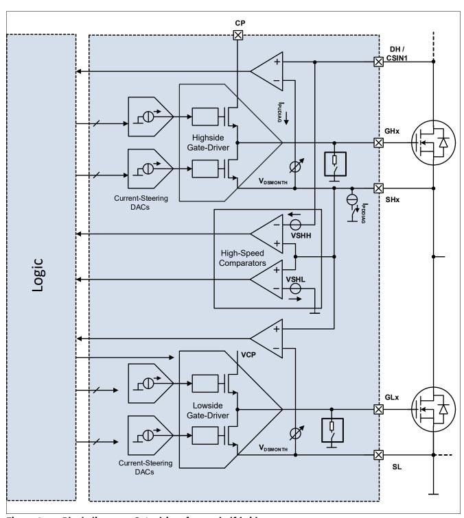
Figure 6 Block diagram - Gate driver for one half-bridge
