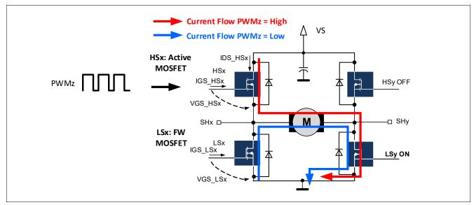
PWM channel z is mapped to high-side x, motor operating as load Figure 16
