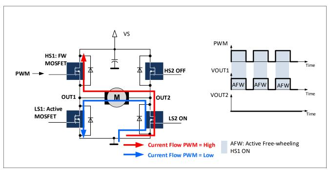
Figure 13 Active freewheeling on HB1: PWM1EN = 1. PWM applied to HS1 (HB1MODE[1:0] = 10<sub>B</sub>). The motor operates as generator: LS1 is the active MOSFET, HS1 is the FW MOSFET.
