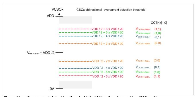
Figure 40 Overcurrent detection thresholds in bidirectional operation (CSDx = 1)
