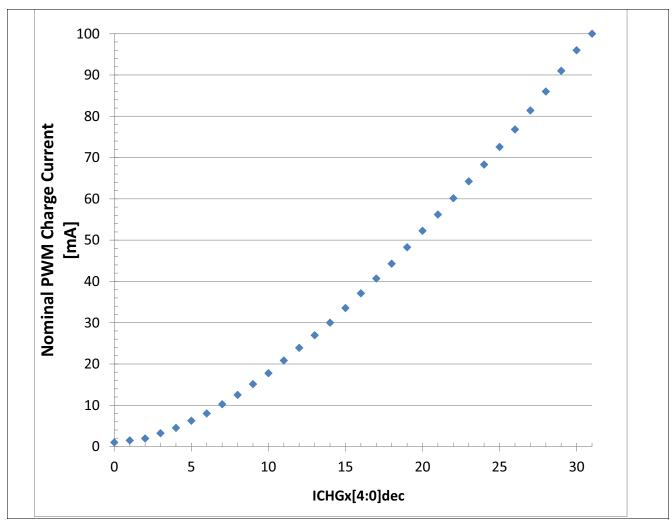
Figure 31 Configurable charge currents in PWM operation
