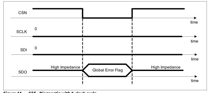
Figure 44 GEF - Diagnostic with 0-clock cycle
