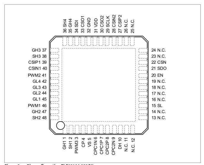
Figure 3 Pin configuration TLE92104-232QX
