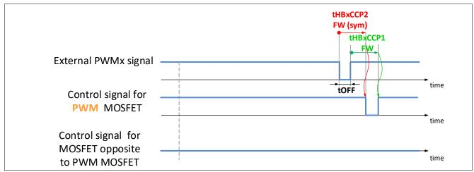
Figure 29 Internal signals for PWM operation at high duty cycle, tOFF < tHBxCCP active
