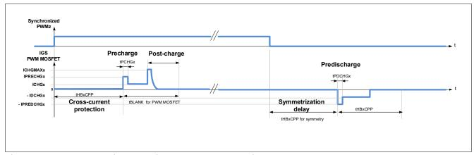
Figure 15 PWM overview showing pre-charge, pre-discharge and post charge phases,  $AGC[1:0] = 10_B$  or  $11_B$ , POCHGDIS =  $1_B$ .
