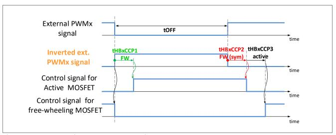
Figure 28 Internal signals for PWM operation - General case: tOFF > tHBxCCP FW, tON > tHBxCCP active, motor operating as generator
