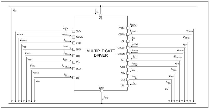
Figure 2 Voltage and current definition
