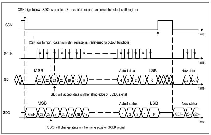
Figure 42 SPI Data Transfer
