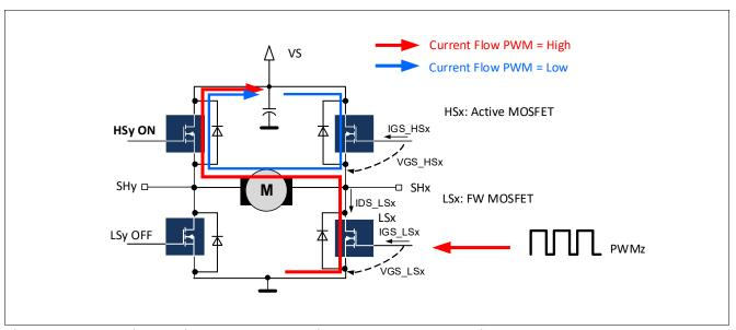
PWM input z is mapped to low-side x, the motor operating as generator Figure 22
