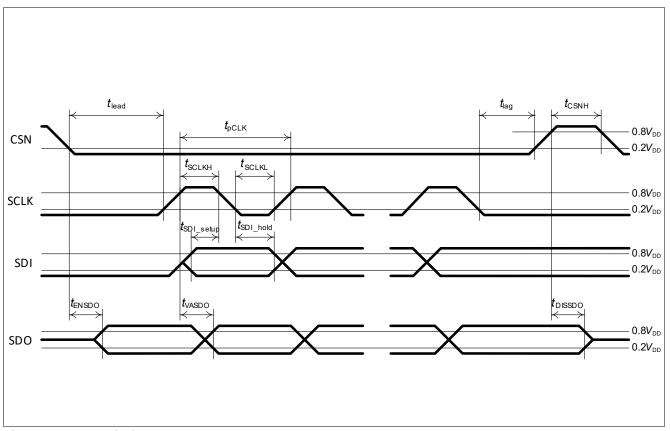
Figure 48 **SPI timing parameters**
