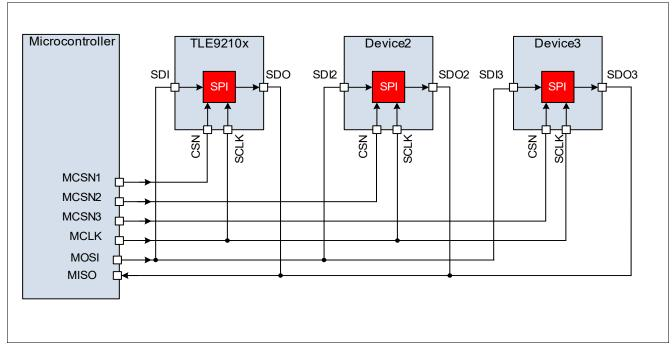
Figure 41 Individual slave selection with three slave devices
