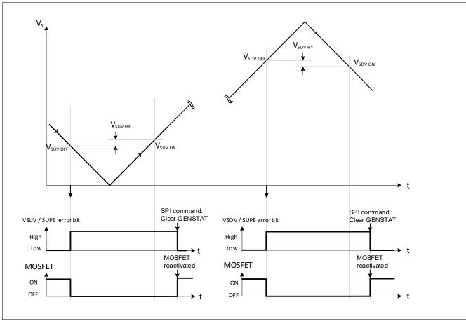
Figure 37 Output behavior during Over- and Undervoltage V<sub>s</sub> condition
