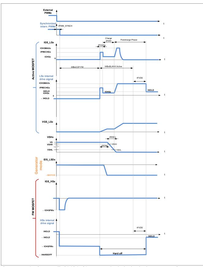
Adaptive turn-off with high-side PWM, AGC[1:0] = (1,0) or (1,1), motor operating as Figure 23 generator
