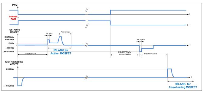
Blank time for half-bridges in PWM operation, detection of generator mode enabled Figure 35 (EN\_GEN\_CHECK = 1), motor operating as generator
