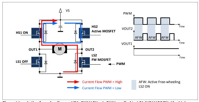
Figure 14 Active freewheeling on HB2: PWM1EN = 1. PWM applied to LS2 (HB2MODE[1:0] = 01<sub>B</sub>). The motor operates as generator: HS2 is the active MOSFET, LS2 is the FW MOSFET.
