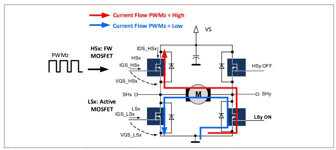
Figure 20 PWM input z is mapped to high-side x, the motor operating as generator
