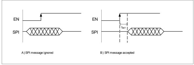
Setup time from EN rising edge to first SPI communication Figure 49
