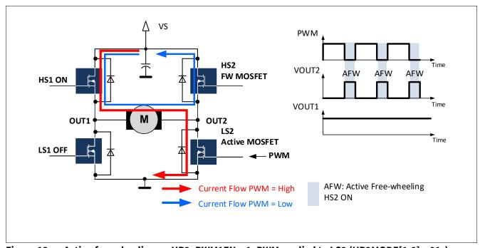
Figure 12 Active freewheeling on HB2: PWM1EN = 1. PWM applied to LS2 (HB2MODE[1:0] =  $01_B$ ). The motor operates as load: LS2 is the active MOSFET, HS2 is the FW MOSFET.
