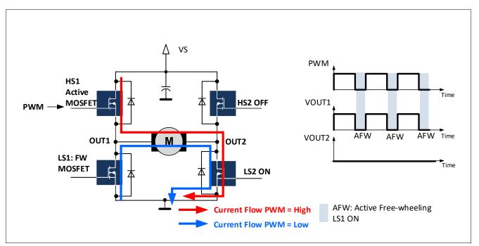
Figure 11 Active freewheeling on HB1: PWM1EN = 1. PWM applied to HS1 (HB1MODE[1:0] =  $10_B$ ). The motor operates as load: HS1 is the active MOSFET, LS1 is the FW MOSFET.
