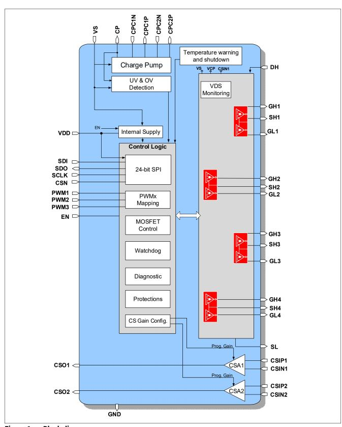
Figure 1 Block diagram
