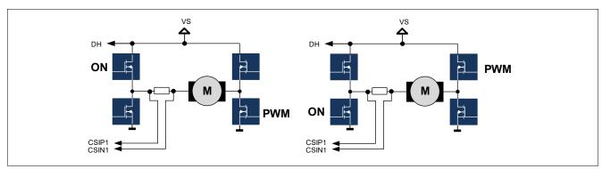
Figure 51 PWM with Shunt resistance in the motor phase
