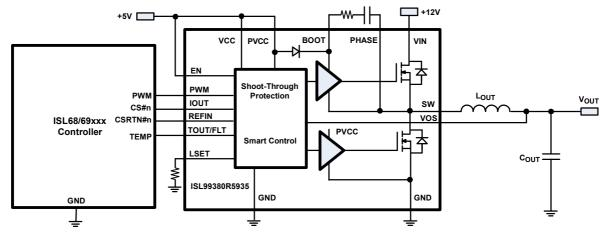
Figure 1. ISL99380R5935 Simplified Application Block Diagram
