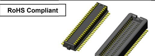
The AC01 series is a 0.5mm pitch horizontal board to board connector, suitable for information and communication equipment, and various other industrial equipment. The connector series are available in 2.5mm and 3.0mm stacking heights, as well as utilizing a highly stable and reliable contact structure which has been proven over decades of use.
