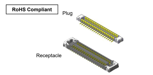
The WP27D Series is a 0.35mm pitch low-profile stacking type board-toboard (FPC) connector with special hold-downs that can be used as power supply terminals, and is ideal for high-density mounting in slim and compact information communication devices like smartphones. This product has a structure that adds protection to the mating surface to prevent damage to the insulator in case force is applied while connectors are misaligned. Also the hold-downs can be used as high-current terminals.
