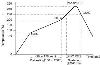
Note: The temperature profile indicates the maximum temperature of the connector surfaces at the highest point from the PCB mounting surface.
