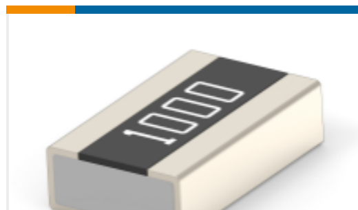
TE Part #2176554-1 3430 A2 Jumper 1k RL
