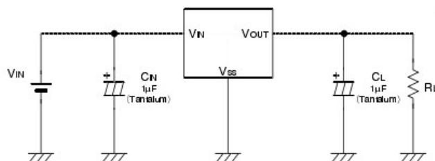
Note1: Input capacitor  $C_{IN}=1\mu F$ .
