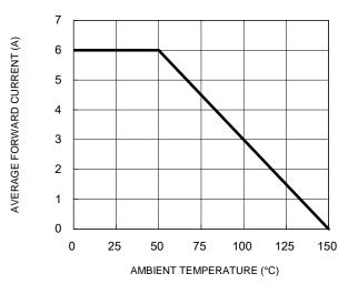
Fig.1 Forward Current Derating Curve
