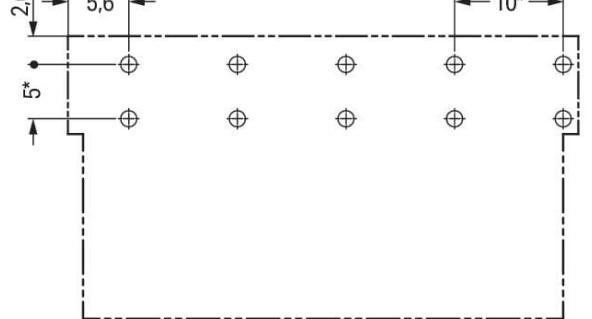
Drilled hole diameter:  $1.5^{+0.1}$  mm
