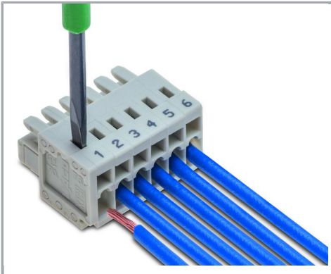
Inserting a conductor via (2.5 x 0.4) mm screwdriver – CAGE CLAMP® actuation perpendicular to conductor entry.
