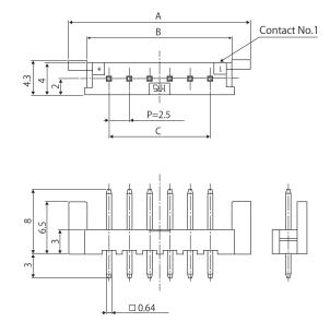
Note : Board Through-hole Diameter :  $\phi$  1.1  $^{+0.1}_{-0.1}$
