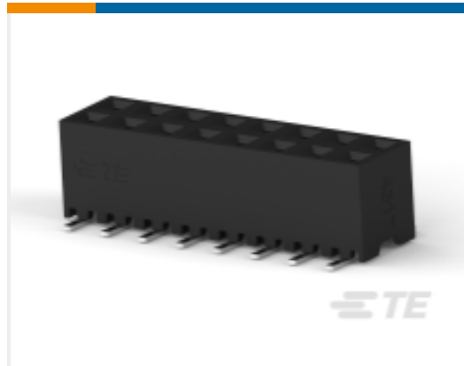
TE Part #1-2314844-6 16P,2MM,B-B,REC,DRVT,SMD,0.1AU, TB,W/CP
