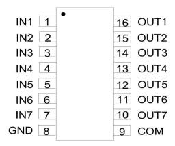
DIP-16/SOP-16/TSSOP-16 (Top View)
