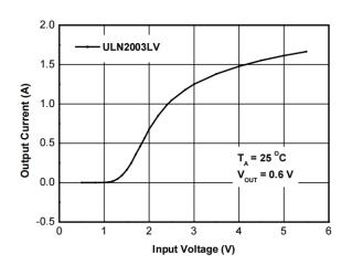
Output Current vs. Output Voltage
