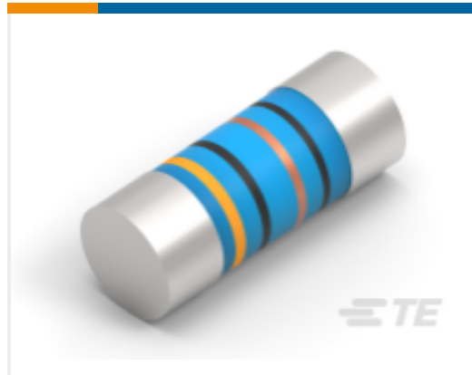
TE Part #2176314-4 MELF SMA_A 180R 0.1% 15PPM 0102 0.3W
