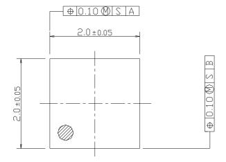
**Terminal Treat** : SnBi Board : Copper **Molding Material** : Epoxy resin Weight : 5.0mg
