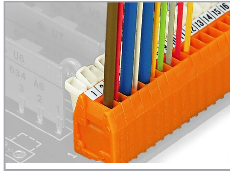
Nominal cross-section: 0.5 mm 2 (20 AWG), 0.75 mm 2 (18 AWG) only in every other position
