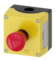
Enclosure for command devices, 22 mm, round, Enclosure material plastic, Enclosure top part yellow, 1 control point plastic, Control point in center, A=EMERGENCY STOP mushroom pushbutton red, 40 mm, rotate-to-unlatch, 1 NC, screw terminal, floor mounting, 1xM20 each on top and bottom
