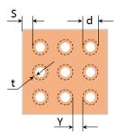
Figure 12 Thermal Via Pattern
