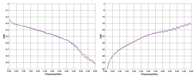
Figure 5 RF1, RF2 Insertion Loss
