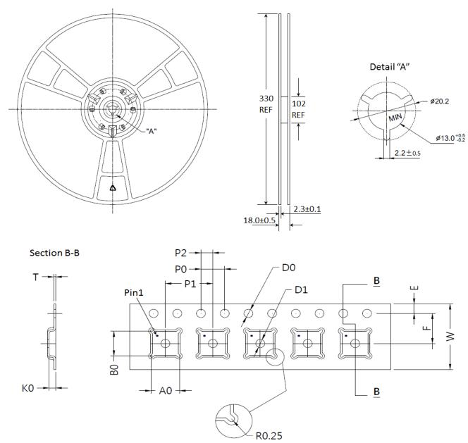
Figure 15 Tape and Reel Drawing
