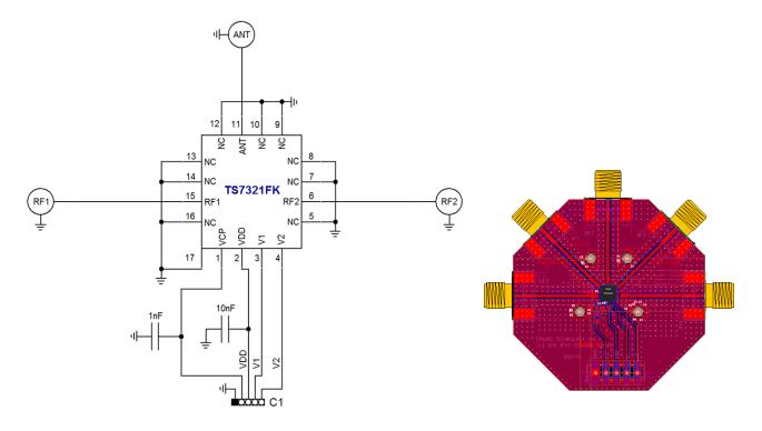
**Figure 3 Evaluation Board Schematic**
