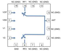
Figure 2 Function Block Diagram (Top View)
