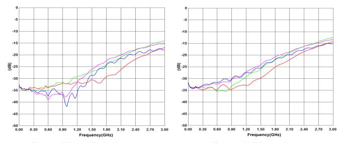
Figure 7 RF1 to RF4 Return Loss
