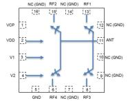
Figure 2 Function Block Diagram (Top View)
