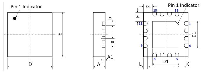
Figure 9 Device Package Drawing
