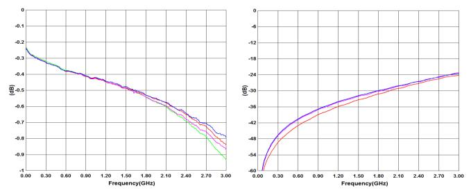
Figure 5 RF1 to RF4 Insertion Loss
