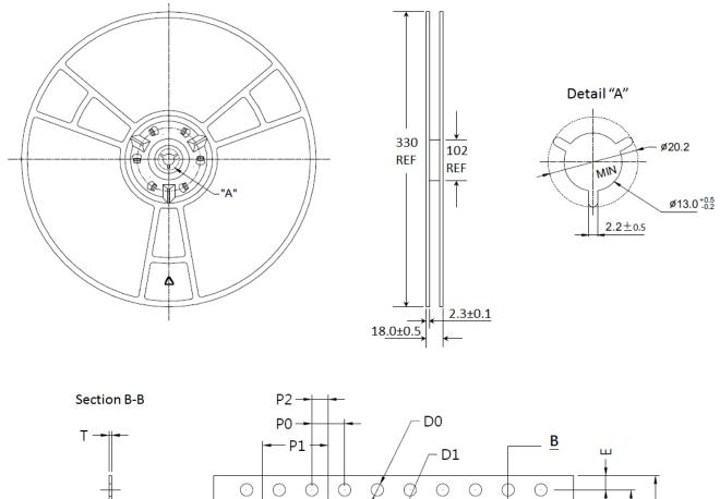
**Figure 15 Tape and Reel Drawing**
