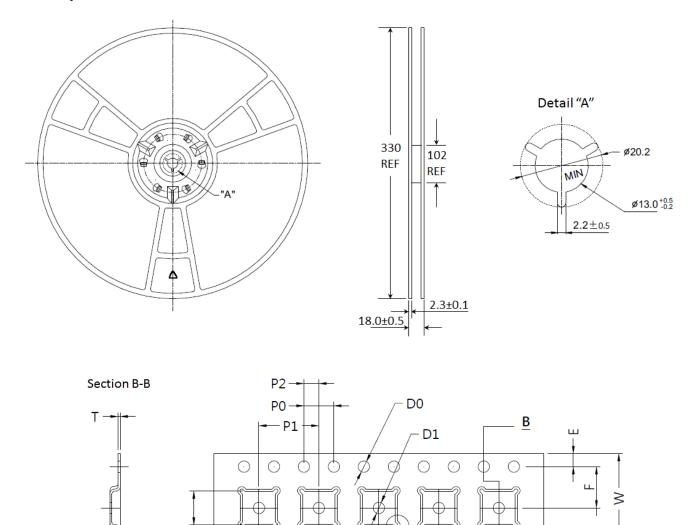
Figure 15 Tape and Reel Drawing
