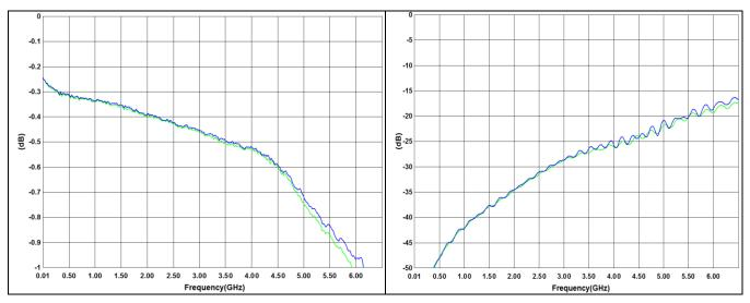
Figure 5 RF1, RF2 Insertion Loss
