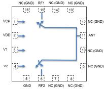
Figure 2 Function Block Diagram (Top View)
