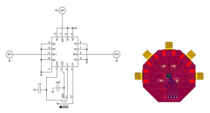
**Figure 3 Evaluation Board Schematic**
