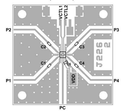
PCB: FR-4, t=0.2mm Capacitor Size: 1005 (1.0 x 0.5 mm)
