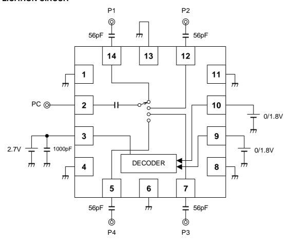
No external DC blocking capacitor at PC terminal is required because of the internal capacitor in IC.
